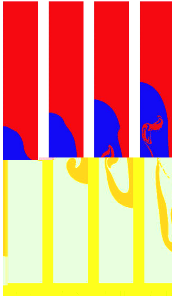
Fig. 17. Evolution of the fluid interface for p = 3 . The Atwood number is 0.5 and the Reynolds number is 500.
